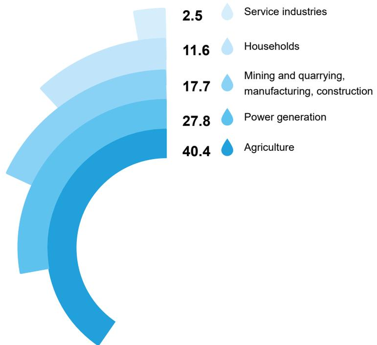
In the case of Poland, power generation is the largest industrial demand for water, accounting for approximately 25% of the country's annual water consumption. Water is primarily used in coal-fired power plants to cool the power units.
