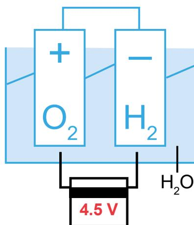
Water is needed to produce green hydrogen, i.e. hydrogen that does not emit CO<sub>2</sub> into the environment. It is the basis of the electrolysis process, during which its molecule is broken down into hydrogen and oxygen when subjected to an electric current. For the reaction to take place, it is necessary to prevent these elements from recombining. A separator placed between the electrodes serves this purpose.
